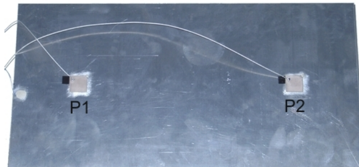
Figure 4: Aluminium plate with two quadratic piezo-electric elements.
